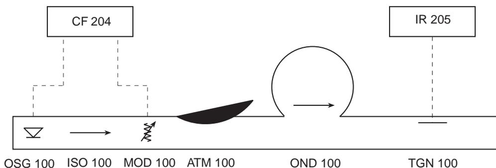
Turn the micrometer screw on the ORITEL OND 100 wavemeter until you obtain an absorption of the microwave energy characterised by a sudden deviation to zero of the galvanometer reading. Read the position indicated by the micrometer screw, with the galvanometer reading being as close as possible to zero.
