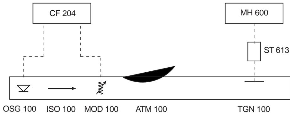
When we do not know the order of magnitude of the power to be measured, it is essential to take certain precautions, in particular so as not to apply a power greater than 200 mW to the measuring probe.
