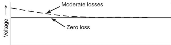
d) Load impedance equal to the characteristic impedance:  $Z_c = Z_0$
